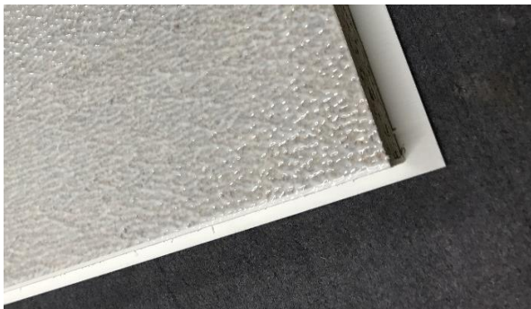
Full surface glue application
